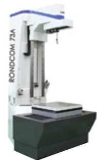
Detector Rotate Roundness Model: R73, R76 Measuring Range: \phi 500\text{mm} Measuring height: \sim 1500\text{mm} Table Size: \sim 800\text{x}600\text{mm} Max. Load: \sim 1000\text{kgs} Rotational Accuracy: (0.04+3H/10000)\mu\text{m}
