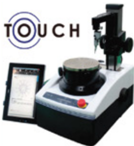
Compact Roundness Model: R-Touch Measuring Range: \phi 150\text{mm} Measuring height: \sim 160\text{mm} Table Size: \phi 148\text{mm} Max. Load: \sim 15\text{kgs} Rotational Accuracy: (0.04+6H/10000)\mu\text{m}
