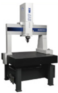
Manual CMM Model: SVF NEX Measuring Range: X 400-1000mm Y 350-2000mm Z 300-600mm Accuracy MPE E (μm): 3.0+4L/1000-
