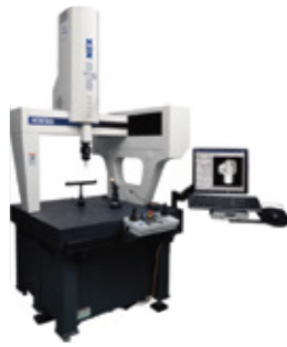
Compact CNC CMM Model: mju NEX Measuring Range: X 510mm Y 460-760mm Z 410mm Accuracy MPE E (μm): 2.2+L/250-
